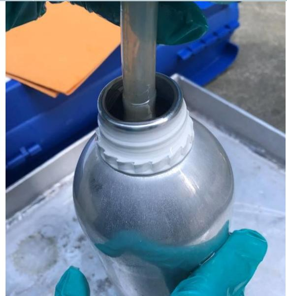
**5** Ending of hose which is linked to valve is placed at the bottom of sampling bottle. Valve is opened slowly to prevent bubbles and filled by starting from bottom of bottle.
