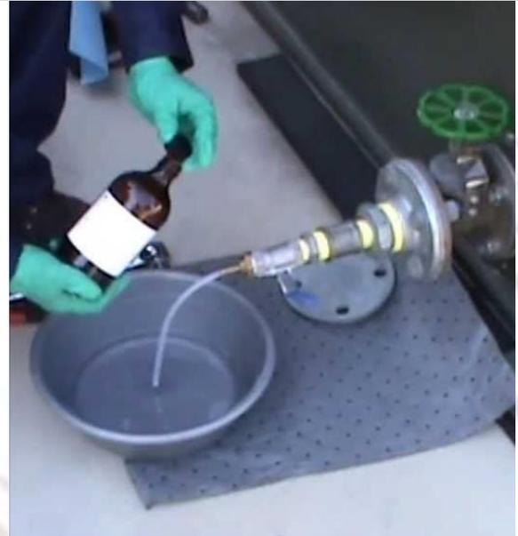
**1** Taking oil sample is inadvisable in rainy weather. If taking the sampling in rainy weather is compulsory, the area must be covered. Sample in glass bottles should not be exposed to the sun.
